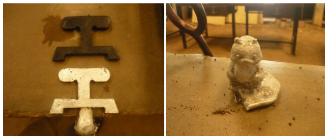
Figure 4. Casting obtained using PLA investment.
