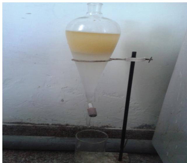
Figure 2 Solution after treatment left in standing funnel for settlement
