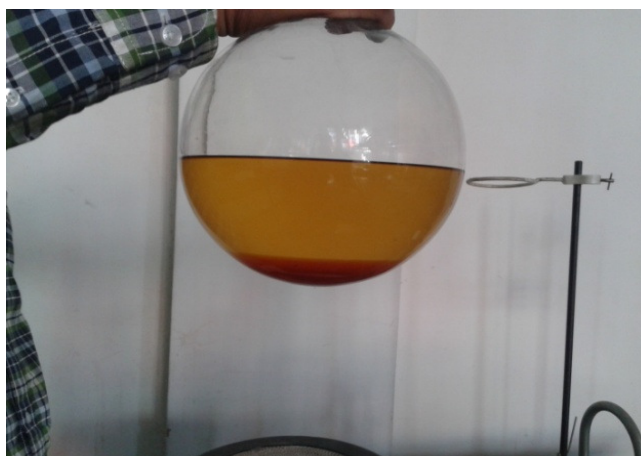
Figure 3 Showing glycerol level at the bottom after the whole reaction process
