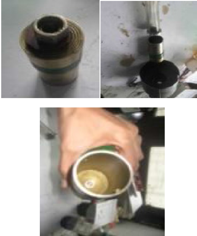
Fig. 6 Trial-3 Modified Redwood viscometer with permanent magnetic strip wound around the viscometer.
