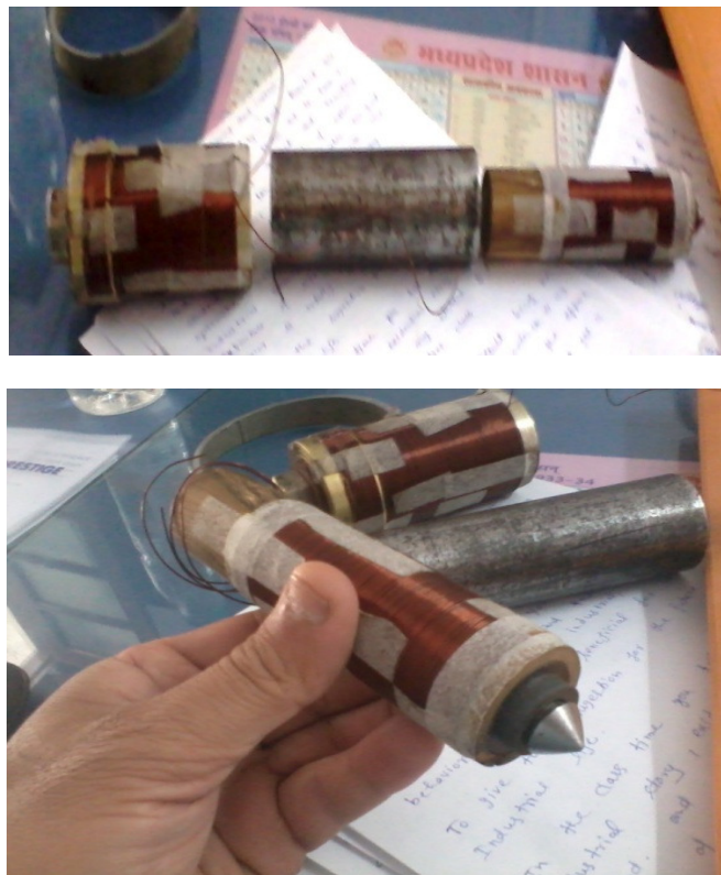
Fig. 5. Trial-2 Modified Redwood viscometer with electrical winding
