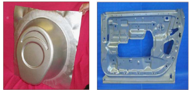
(a) (b) Fig. 1: Typical applications of superplastic forming (a) Aerospace Component (b) Automotive door panel [1]
