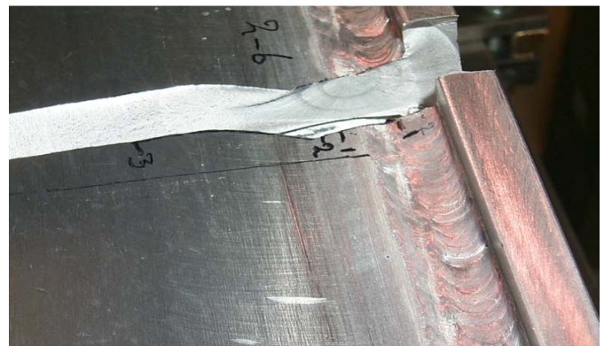
Figure 1 Fatigue Crack in Aluminium
