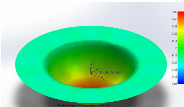
**Fig. 4- Thickness distribution in 3mm blank**
