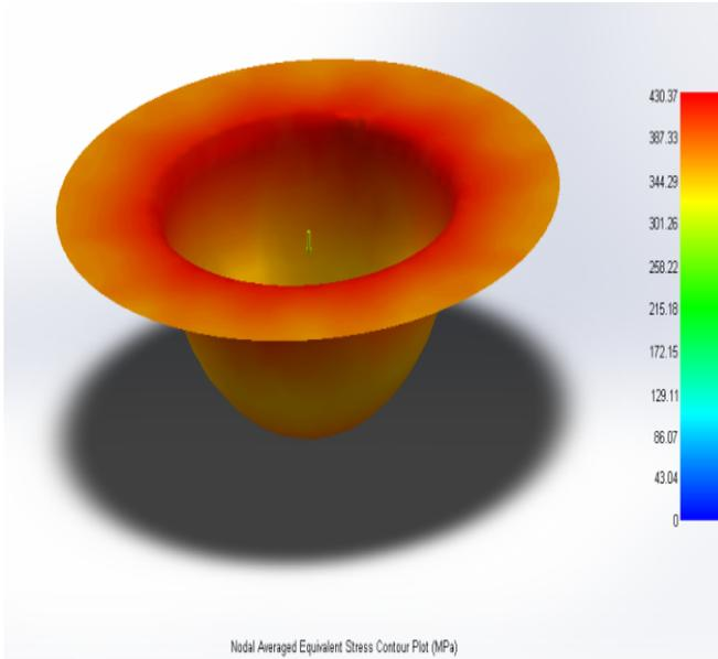
**Fig. 8- Stress distribution in 4mm thickness blank**
