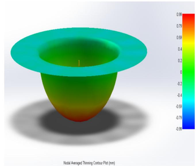
**Fig. 10- Thickness distribution in 5mm blank**
