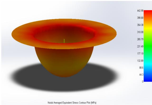
Fig. 11- Stress distribution in 5mm thickness blank
