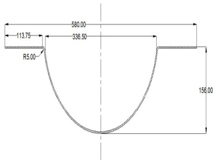
Fig. 15- Geometrical Model of 3mm steel
