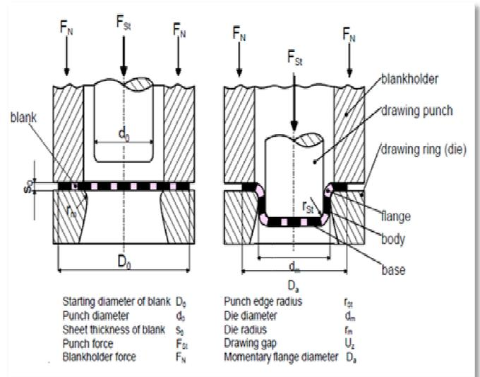
Fig. 1: Deep Drawing Process
