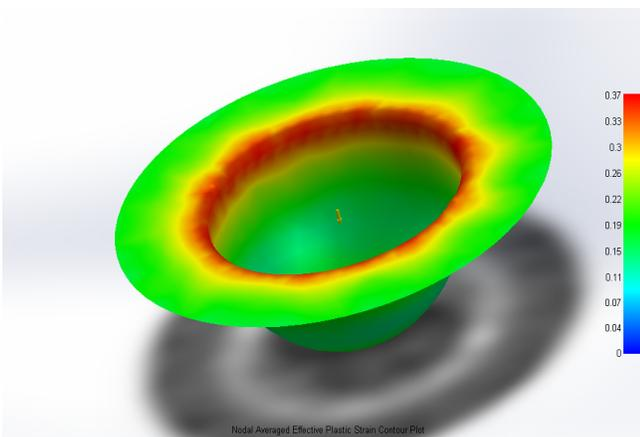
Fig. 12- Equivalent Plastic Strain in 5mm thickness blank
