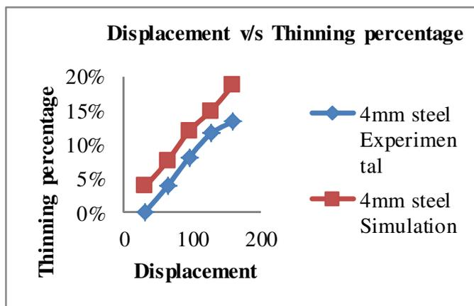
Fig. 19 Validation for 4mm thickness blank (Displacement v/s Thinning percentage)
