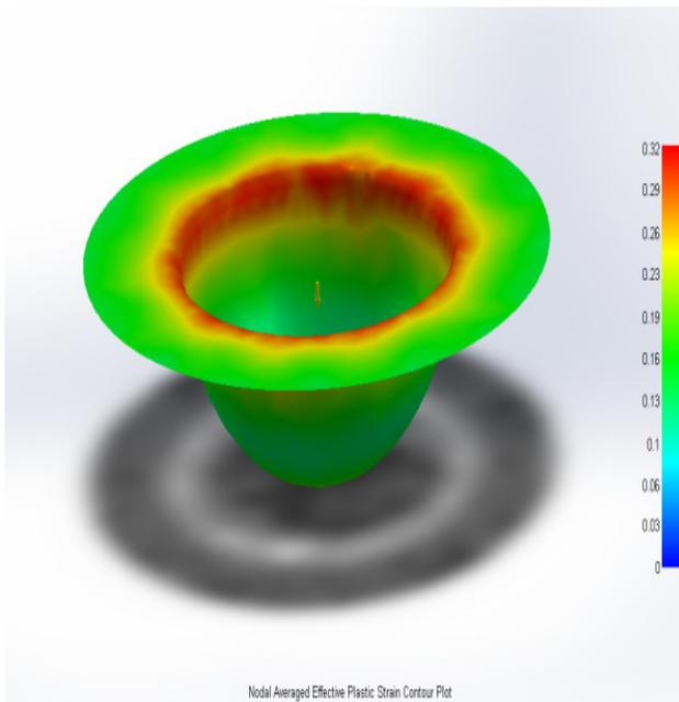
**Fig. 9- Equivalent Plastic Strain in 4mm thickness blank**
