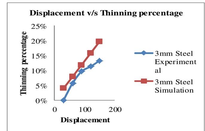
**Fig. 18 Validation for 3mm thickness blank (Displacement v/s Thinning percentage)**
