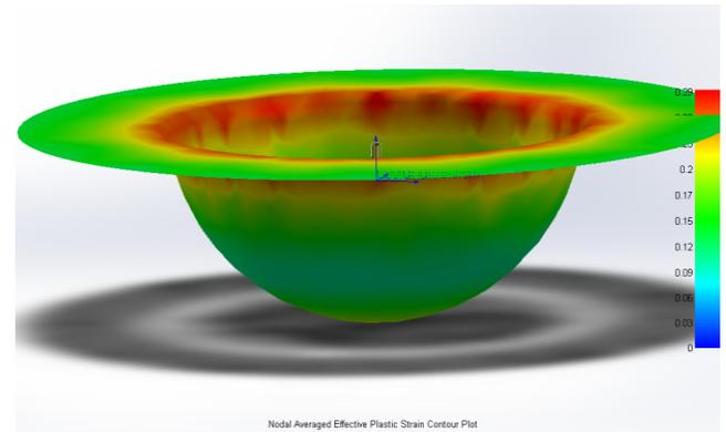
**Fig. 6- Equivalent Plastic Strain in 3mm thickness blank**
