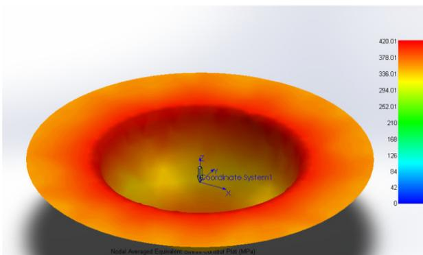
**Fig. 5- Stress distribution in 3mm thickness blank**
