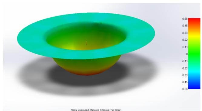
**Fig. 7- Thickness distribution in 4mm blank**
