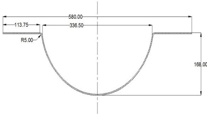
**Fig. 16- Geometrical Model of 4mm steel**
