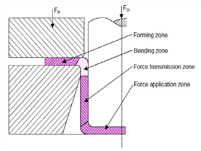
**Fig. 2 Stress Zones During Deep Drawing**
