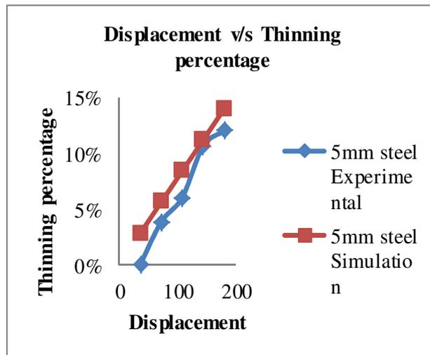
Fig. 20 Validation for 5mm thickness blank (Displacement v/s Thinning percentage)
