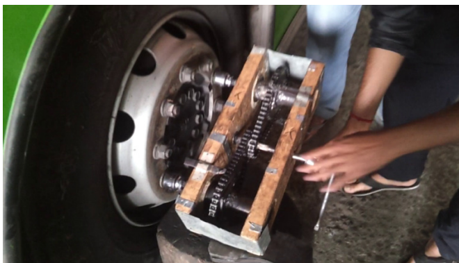
Fig. 2 Testing EMW tool working on DTC low floor bus
