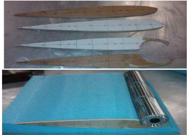
Fig 3.1 Wooden templates of the airfoil profiles
