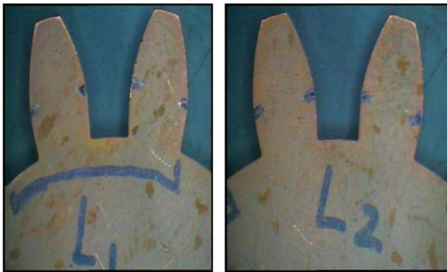
**Figure 3. Microscopic image of copper plate after cutting at 10 X optical zoom.**
