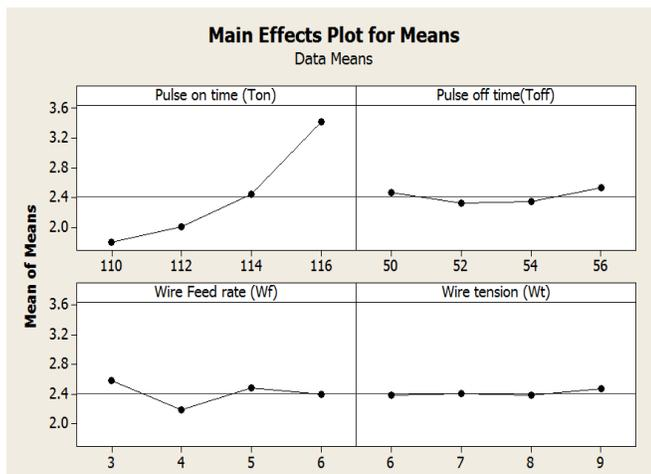
**Figure 4(a).** Main effect plot diagram for variation of different input parameters with MRR.
