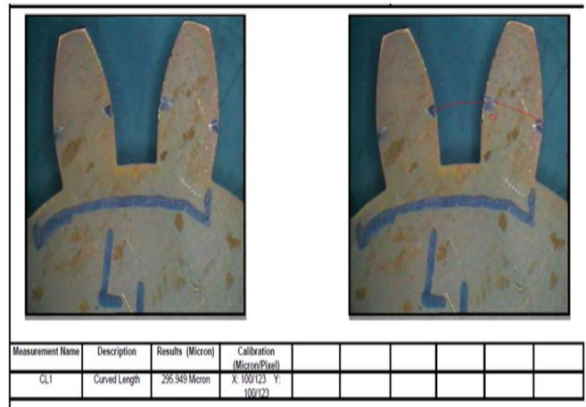
**Figure 3(b). Measurement of actual Pitch error right flank using Caliper pro software.**
