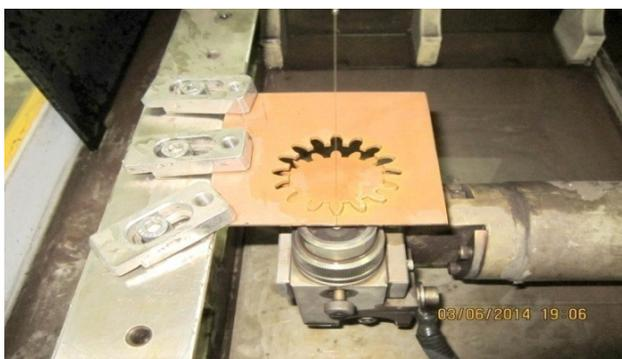
**Figure 2. Machining of copper plate having sixteen number of teeth.**
