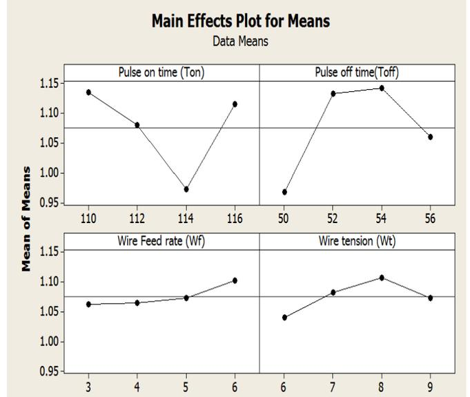
**Figure 4(b).** Main effect plot diagrams for variation of different input parameters with pitch deviation.
