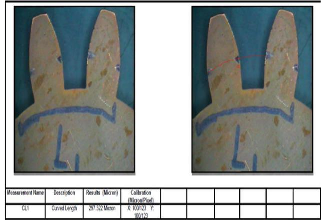
**Figure 3(a). Measurement of actual Pitch error of left flank using Caliper pro software.**
