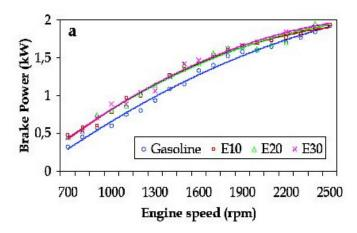
The above graph indicates the influence of ethanol gasoline blended fuels on engine power. When the ethanol content was slightly increased in the blend, the engine brake power slightly increased for all engine speeds. With an increase in the ethanol percentage, the density of the blend increased and the volumetric efficiency increased, increasing the brake power.
