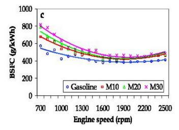
BSFC is defined as the ratio of the rate of fuel consumption and brake power. The energy content of the blend decreases with increase in methanol content. This causes the Brake power to reduce ultimately resulting in increase in BSFC. As the engine speed increases, the BSFC decreases.
