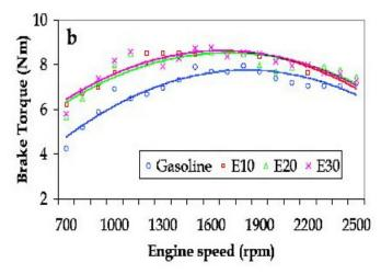
The above graph indicates the influence of ethanol gasoline blended fuels on engine torque. The increase in ethanol content increases the torque slightly. The brake torque of gasoline was lower than E10 and E30, especially due to the addition of ethanol the anti-knock characteristics improved allowing advanced ignition timing which resulted in a higher combustion pressure and thus higher torque.
