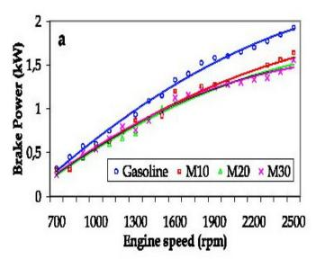
The above graph indicates the influence of methanol gasoline blended fuels on engine power. When the methanol content was slightly increased in the blend, the engine brake power slightly decreased for all engine speeds. The brake power of gasoline is higher than all those methanol blends M10 - M30, especially for high engine speeds at about 2500 rpm. This may be attributed to the slow burning of methanol.
