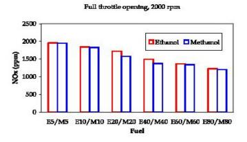
$NO_X$  are usually formed when the temperature within the combustion chamber is very high. Since, ethanol/methanol have higher latent heat of vaporization, the temperatures in the cylinder are maintained at a lower temperature. Hence,  $NO_X$  are reduced.
