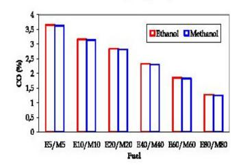
CO is a toxic gas. It is produced as a result of incomplete combustion of gasoline. When methanol or ethanol is blended with gasoline, the amount of CO emission is reduced. This reduction in CO emissions can be attributed to the presence of oxygen in alcohols. You can see from the graph that as the percentage of alcohol in an alcohol-gasoline blend is increased, CO emissions are reduced.
