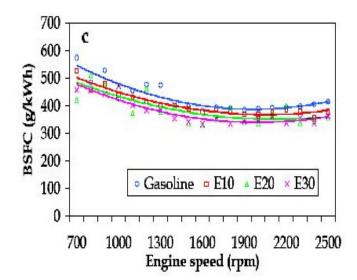
BSFC is defined as the ratio of the rate of fuel consumption and brake power. BSFC decreases as the ethanol content increases. As the engine speed increases, the BSFC decreases. This is due to the increase in brake thermal efficiency.
