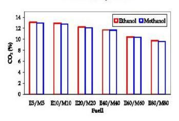
From the above graph, the  $CO_2$  are lower for higher percentage of alcohol in alcohol-gasoline blends. Since, methanol and ethanol have less number of carbon atoms, the amount of  $CO_2$ released will be less compared to the combustion of pure gasoline.
