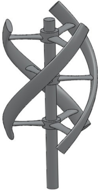
Fig. 3.2. VAWT-3D Cad Model
