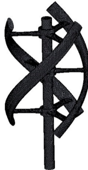
Fig. 4.1. VAWT model mesh by SOLIDWORKS
