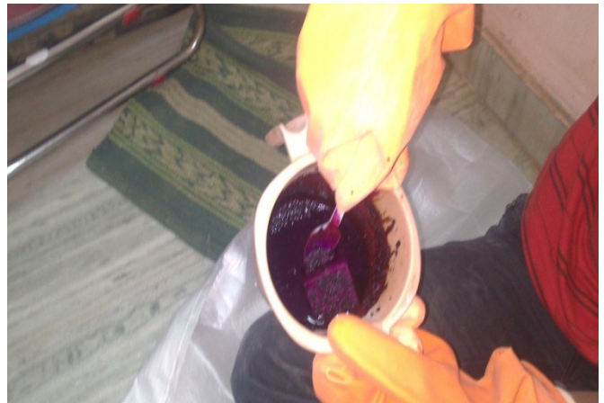
Fig. 4 ceramic filter is dipped into the paste
