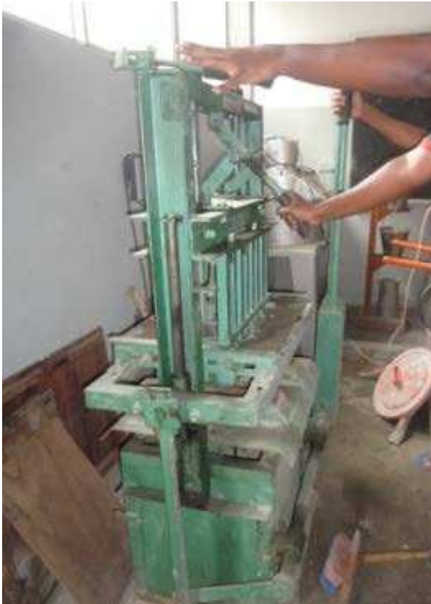
Figure 1: Making of the interlocking paving block in progress
