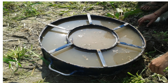
Fig.1 Double Ring Infiltrometer (NIT, Kurukshetra)
