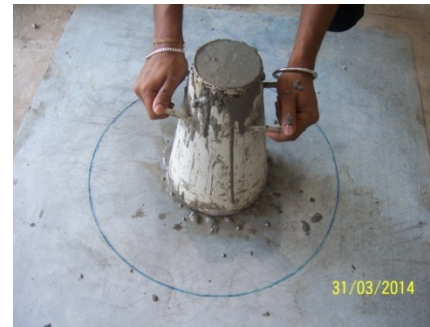
Figure 3. T 500 test of SCC
