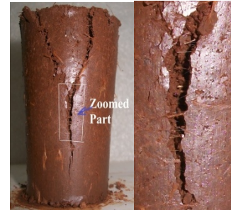
Figure 16. Bridging effect of fibre-reinforcement (0.5%, 20 mm)
