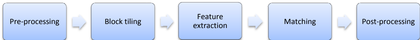
Fig.2. Steps for detection of copy-move forgery
