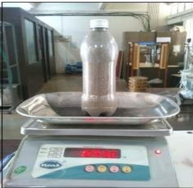
Fig. 2. Weighing balance to weigh Sealed PET bottle before testing
