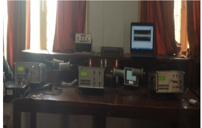
Figure 3.1. Complete Hardware Set up for a Wireless Data Logger Using Satellite Communication System.
