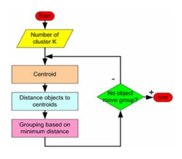
Fig. 5. K-means clustering process
