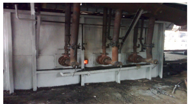
Fig. 3: Producer gas burner installed in soaking zone of furnace
