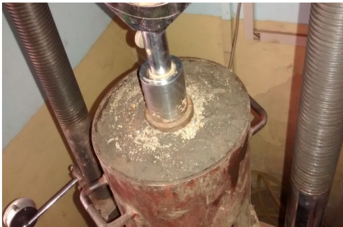
Figure-4: Load test on sand column
