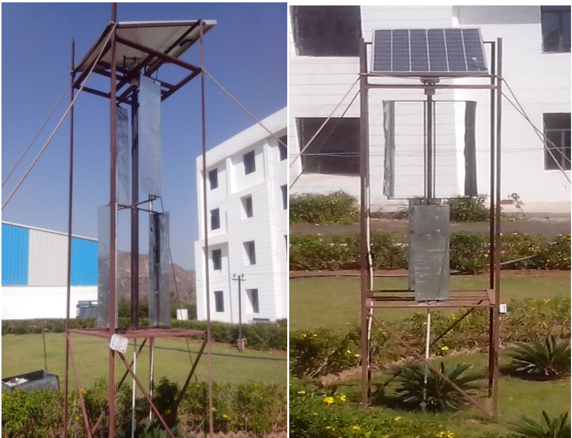
Fig 2: Double stage hybrid wind turbine used for present study
