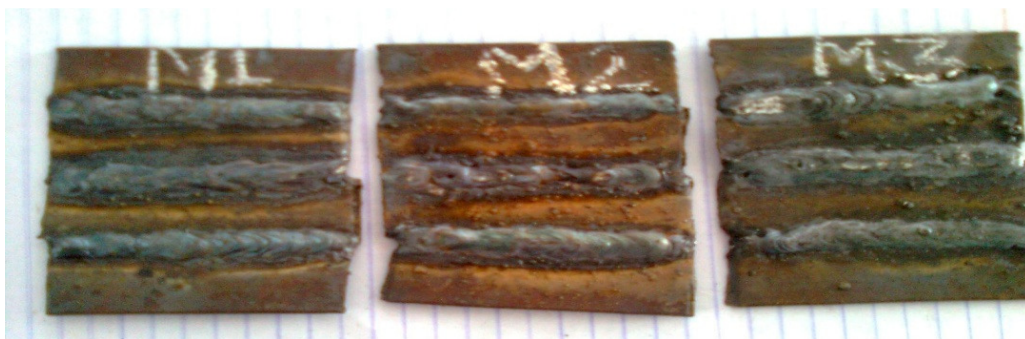
Fig.2 welds joints obtained under magnetic field.
