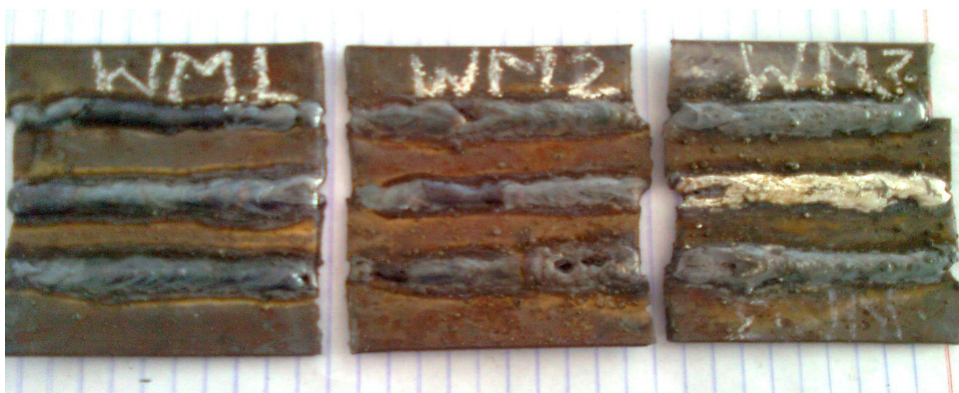
Fig 3 weld joints without magnetic field
