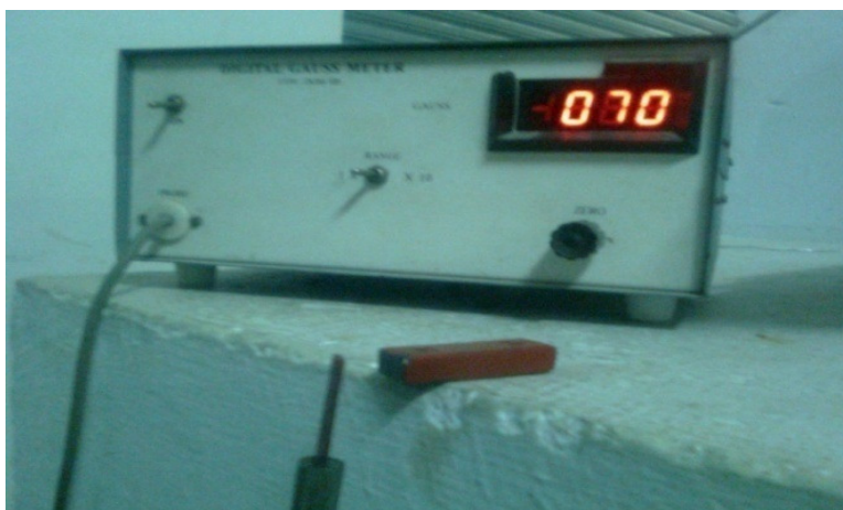
Fig.1- Measurement of magnetic field by Gauss-meter
