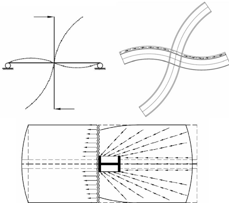
**Figure 2. Composite beam under lateral loads and related slab force transfer mechanism**
