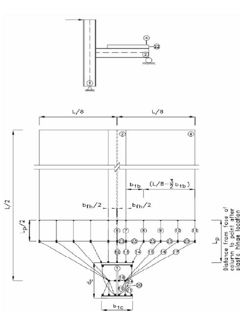
**Figure 8. Second finite element model components**
