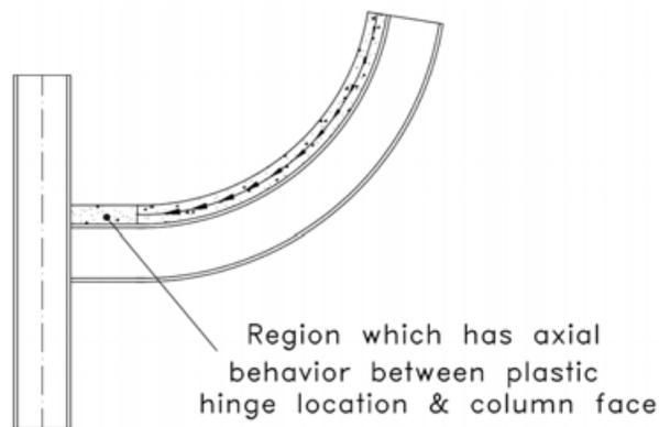
**Figure 3. Exaggerated deformation of a composite beam in positive moment**
