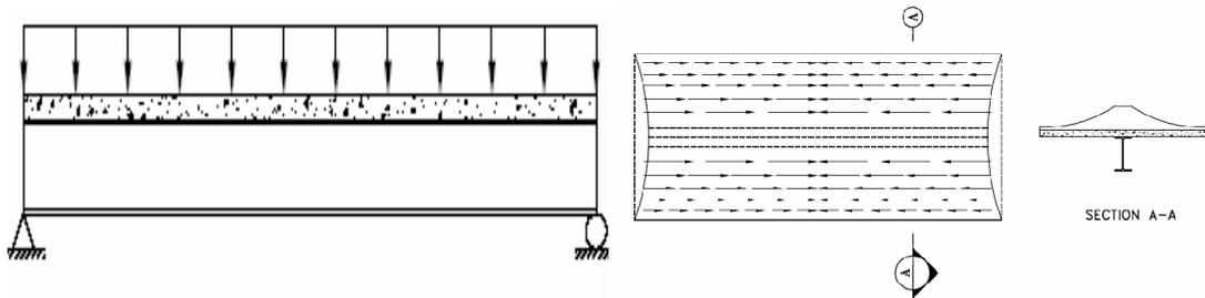
**Figure 1. Composite beam under gravity loads and related slab force transfer mechanism**
