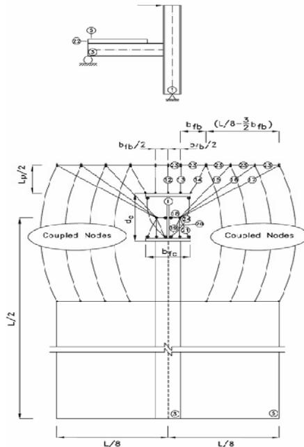
**Figure 9. Third finite element model components**
