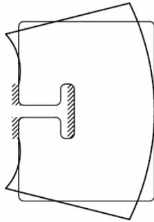
**Figure 6. Slab axial zone deformed shape**
