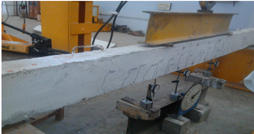
Fig 3: Bonded GFRP beam where tested under four-point load
