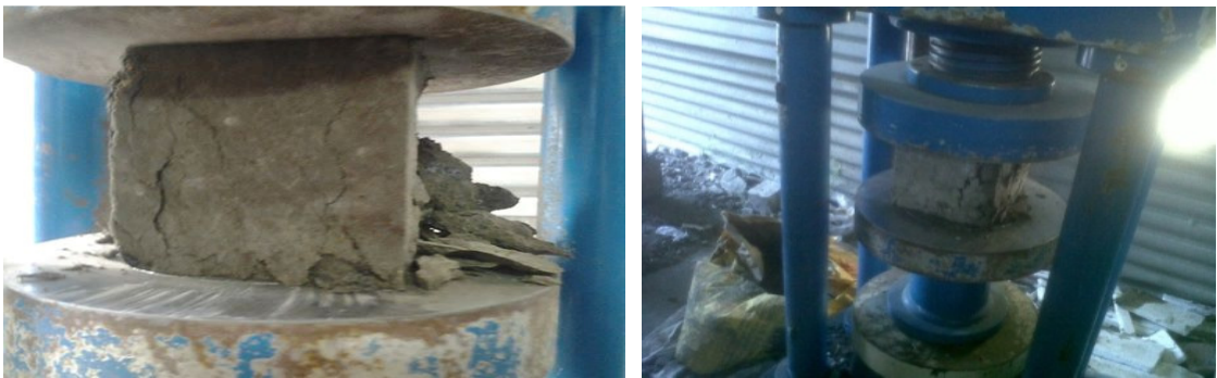
Fig.2. Compressive testing of cubes
