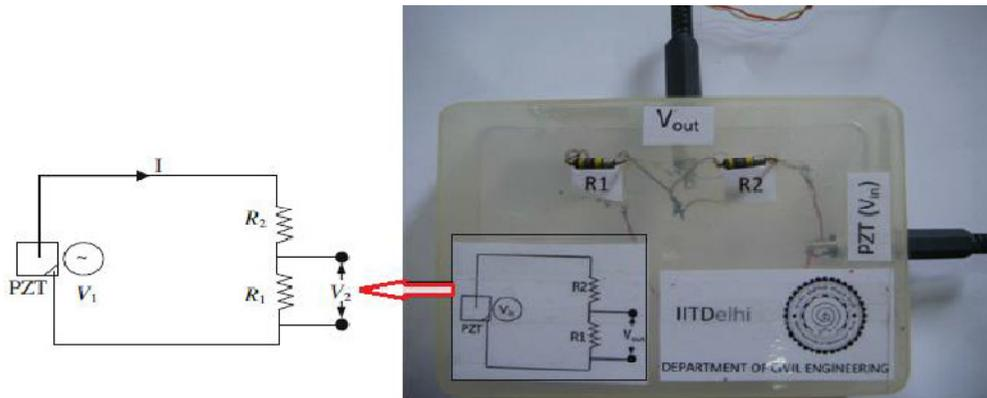
**Fig. 2, Power Measuring Circuit, With Circuit Diagram [2]**
