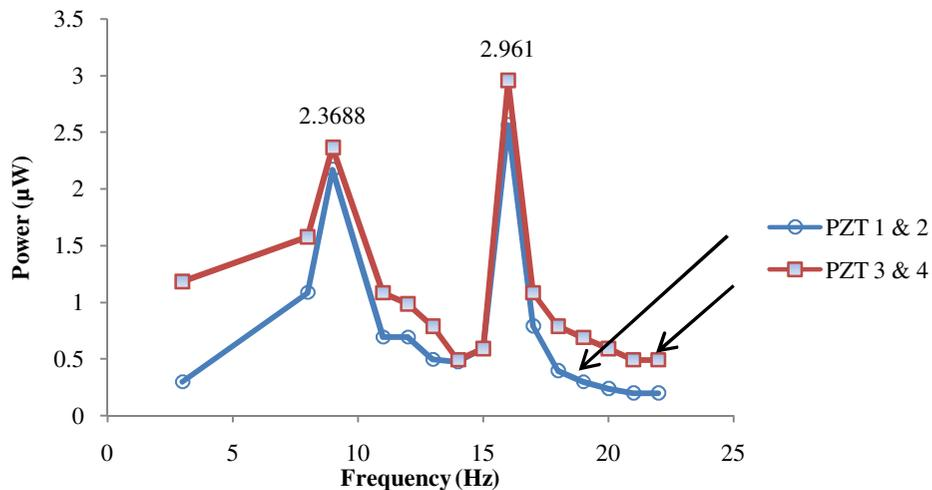
**Fig. 3, Power vs Frequency plot for a single PZT**
