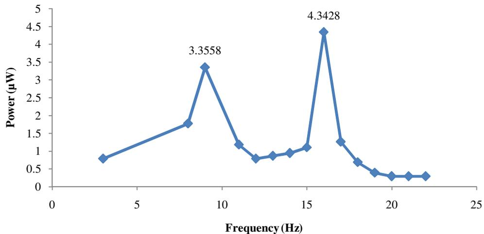
**Fig. 4, Power Vs Frequency plot for a PZT's connected in parallel**
