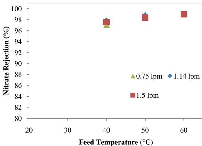
Fig. 2: Effect of feed bulk temperature on nitrate rejection.
