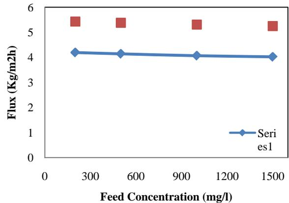
Fig. 6: Model validation for permeate flux in VMD
