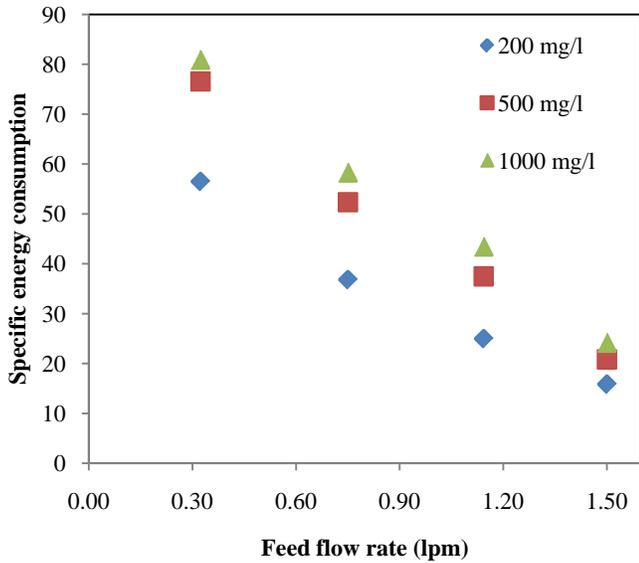
Fig. 5. Effect of feed flow rate on energy consumption.
