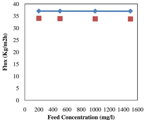
Fig. 8: Model validation for permeate flux in VMD
