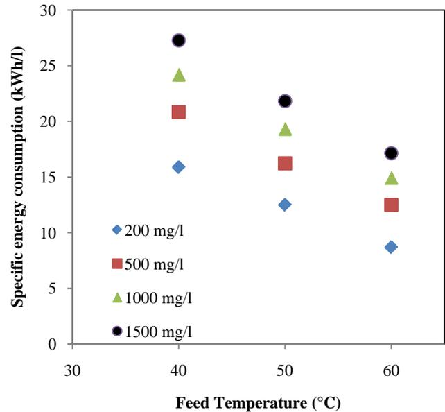
Fig. 4: Effect of feed temperature and nitrate concentration on energy consumption.
