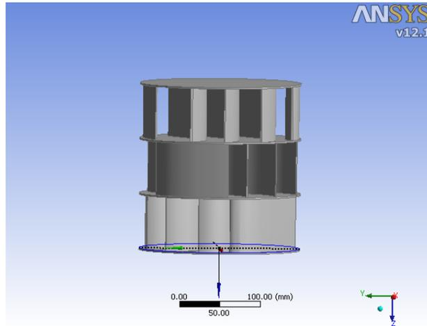
**Fig No. 1 Geometry of three story VAWT**
