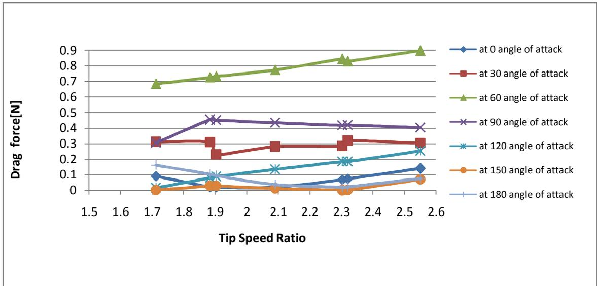
**Fig no 5: Plot of Drag force vs Tip speed ratio for different angle of attack.**
