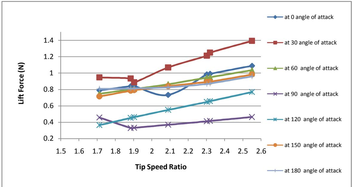
**Fig no 4: Plot of lift force vs. tip speed ratio for different angle of attack.**
