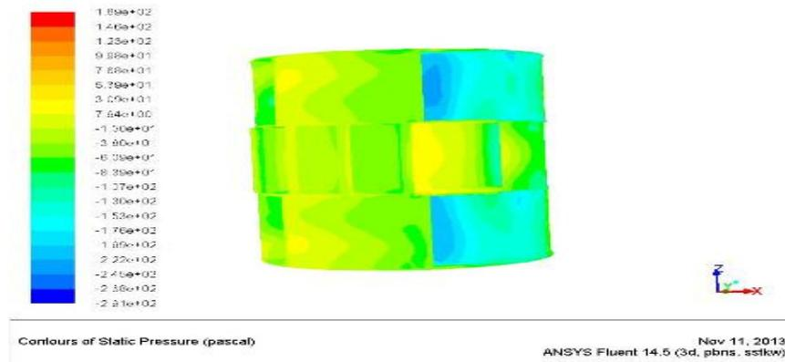
**Fig no 8: Static pressure plot of M VAWT at 0° angle of attack**
