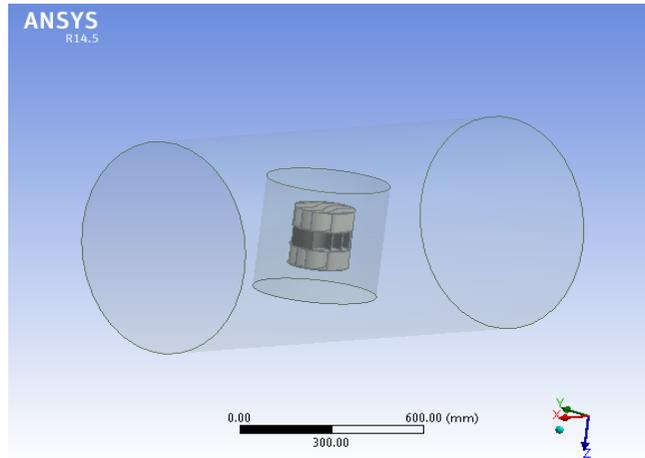
**Fig no 2: Turbine model placed in Moving Reference Frame and Stationary Computational Domain.**
