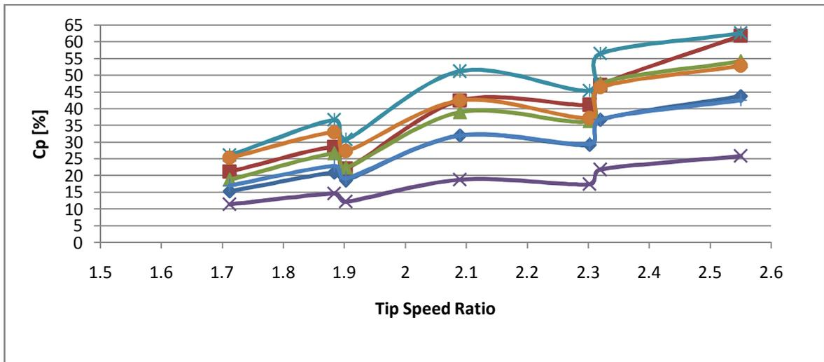
**Fig no 6: Plot of CpVs Tip sped ratio for different angle of attack**
