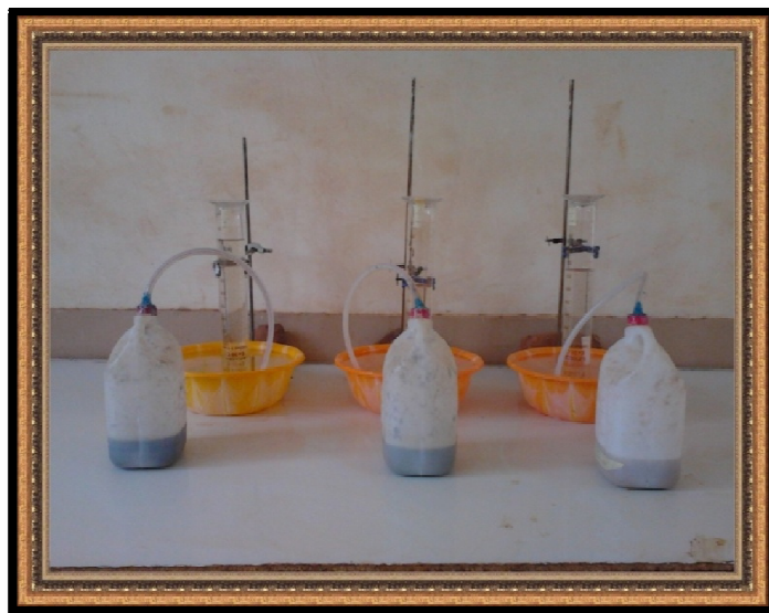
Fig. 1: Bio-methane generation from abdominal waste of Cow, Sheep and Goat (left to right)
