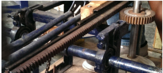
Fig. 5 rack and pinion setup
