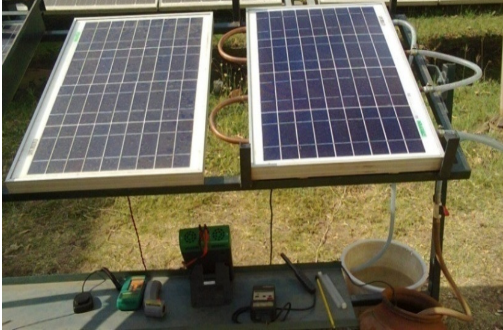
Figure 1: Experimental setup of PV and PV/T system
