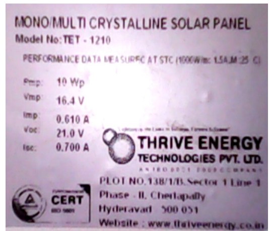
Figure 4: Label of solar panel.
