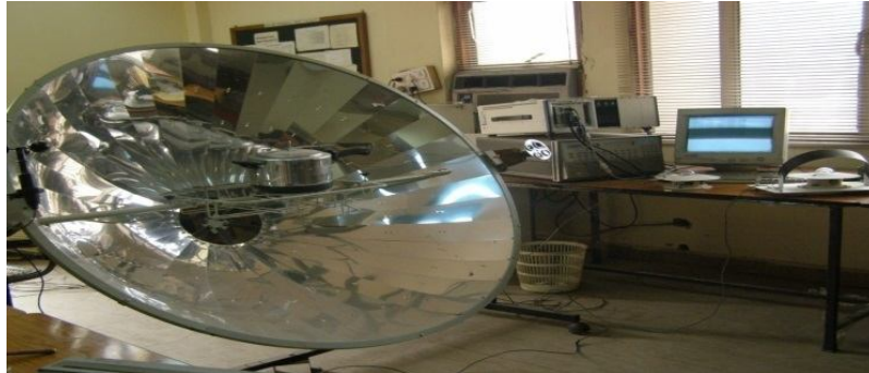
Fig. 4: cooking pot with parabolic dish, for heating test.
