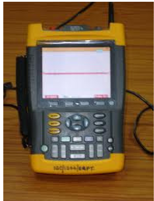
Fig. 2. digital storage Scope Meter (Injection and Combustion Pulses).
