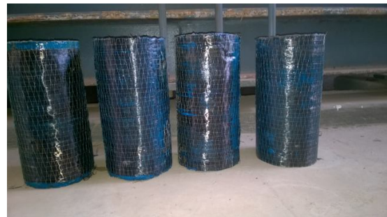
Fig 6. After applying FRP sheets and After curing
