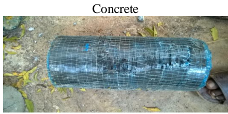
Fig 8. Specimen after applying tensile load
