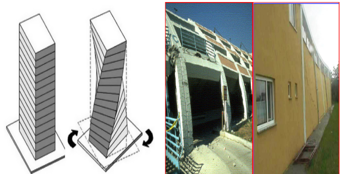
Fig. 1. Failure of irregular structure
