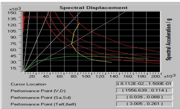
Fig. 11. Performance point for 'C' shaped building
