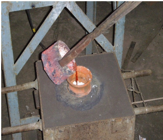
Figure 1: Molten metal poured in to mould
