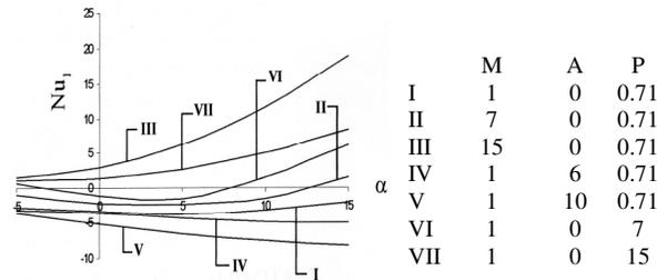
Fig. 8: Heat transfer coefficient  $Nu_1$  at  $y = 1$  against  $\alpha$  when  $m = 2, G = 10, \lambda_x = 0$
