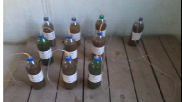
Fig. 2: Lab scale 1L digester set up
