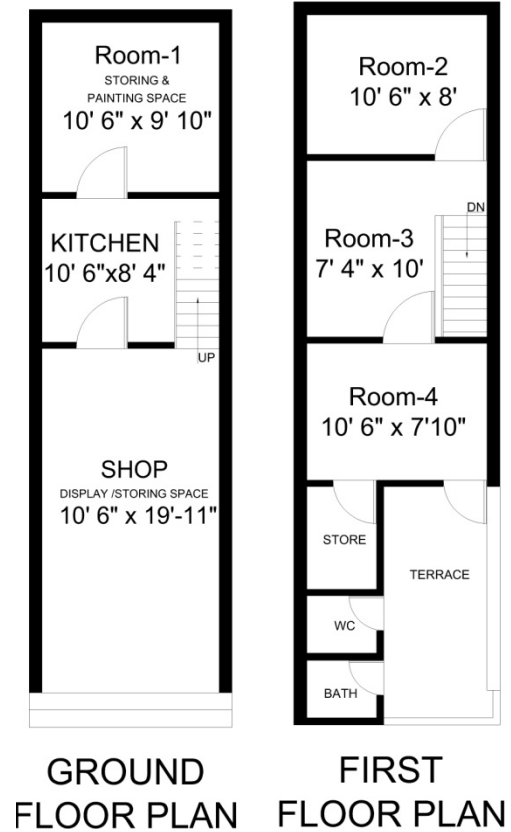
Fig. 5: Floor Plans of Dwelling Unit - 2
