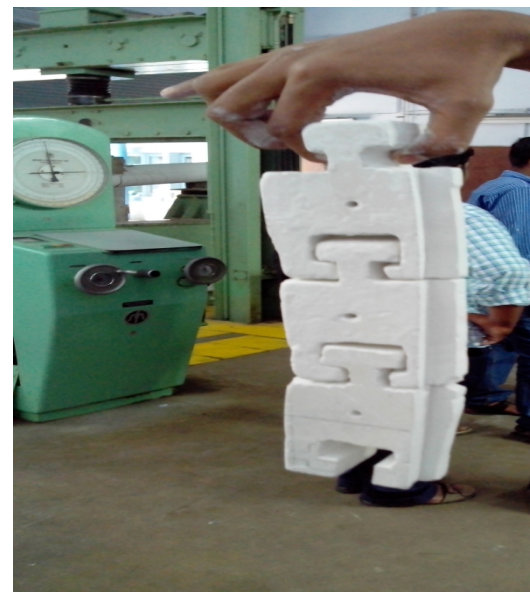
Fig.2 shows the ‘T’ projection in the model of interlock block that we did at ( iitmadras)
