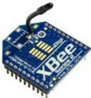
Figure 3. Xbee S2C radio transceiver
