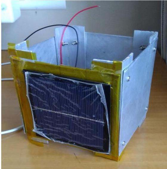
Figure 5.5 Aluminum CubeSat structure
