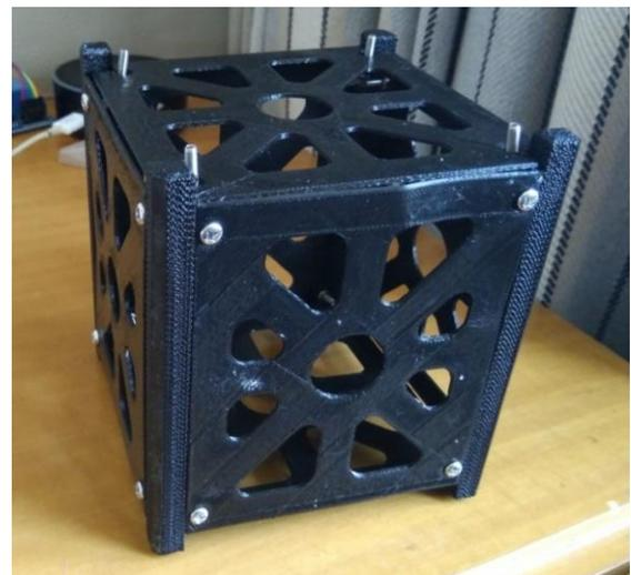
**Figure 5.4 3D printed CubeSat structure**
