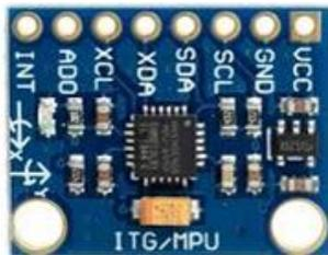
Figure2.2. MPU6050 IMU
