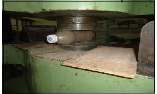
Fig. 3. Test applied on a waste PET bottles filled with soil and sealed tightly
